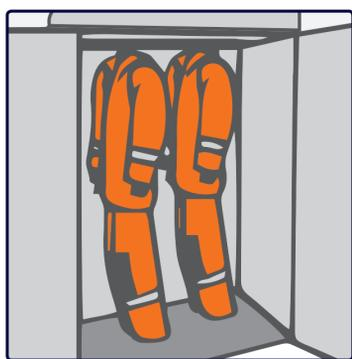
**1** It's a good idea to hang the parts of your work outfit on the same hanger. Begin by hanging the trousers, and then hang the jacket. Then slide in the hanger onto the proper opening in the ceiling of the drying cabinet.
